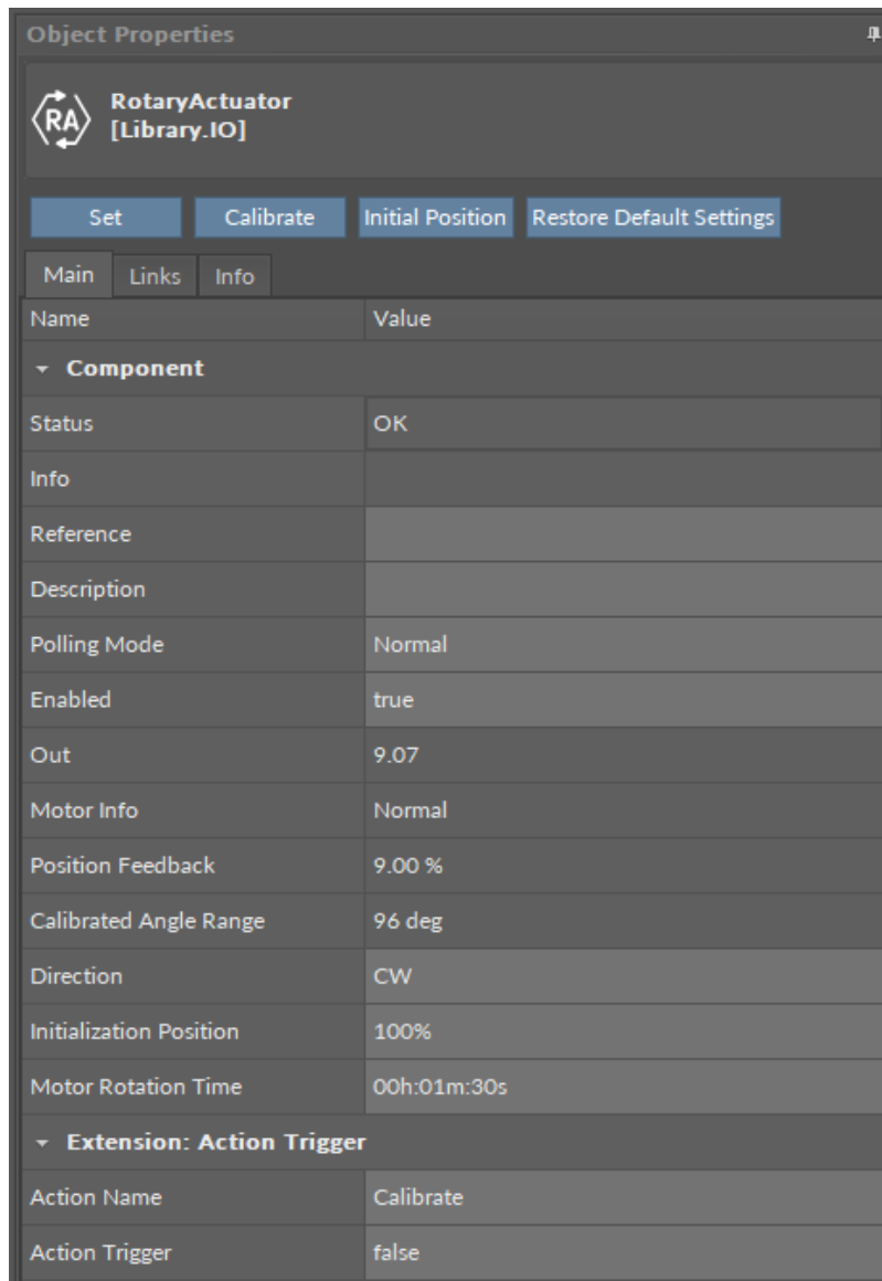
Figure 119. ActionTrigger extension in the RotaryActuator component
