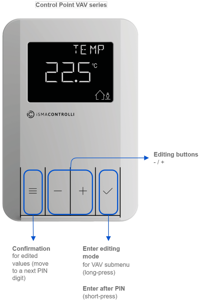
Figure 41. Panel access to the VAV submenu
