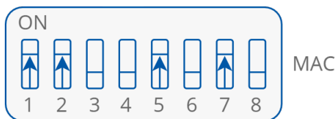
Figure 9. MAC DIP switch settings
