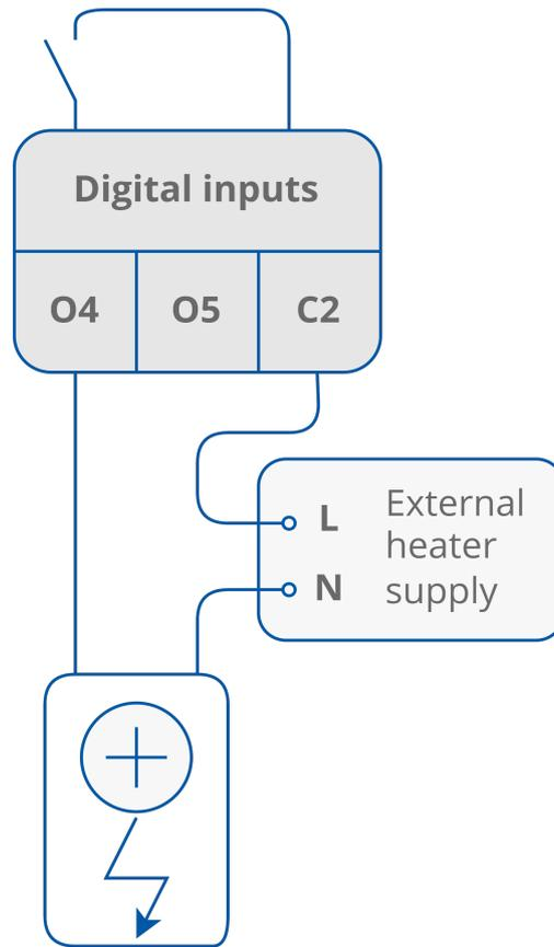
Figure 6. Electrical heater connections
