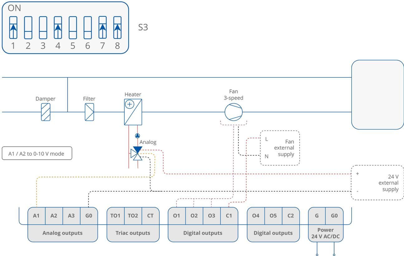
Figure 58. 2-pipe installation with 1-stage analog controlled heating and 3-speed fan - valve in analog mode
