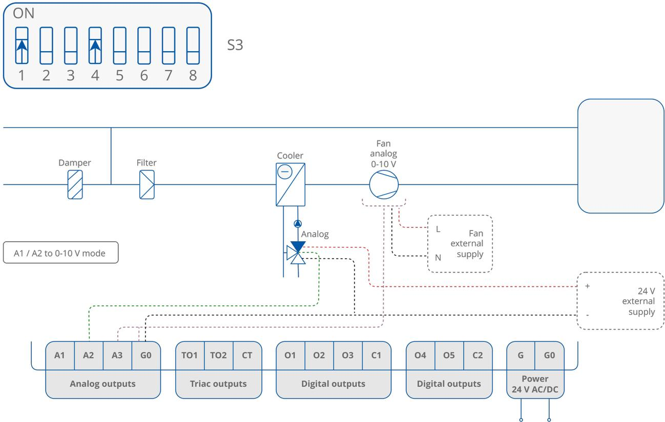
Figure 52. 2-pipe installation with 1-stage analog controlled cooling and analog controlled fan - valve in analog mode
