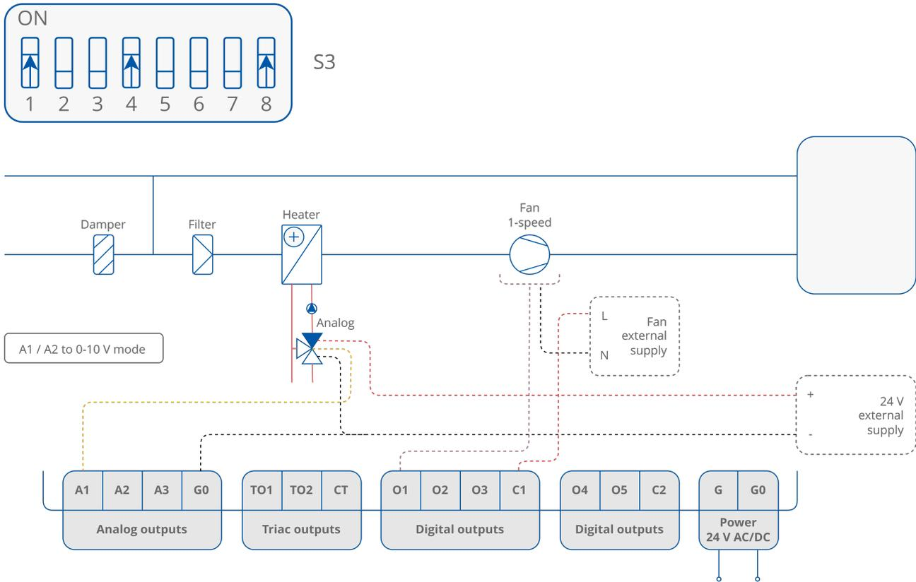
Figure 54. 2-pipe installation with 1-stage analog controlled heating and 1-speed fan - valve in analog mode
