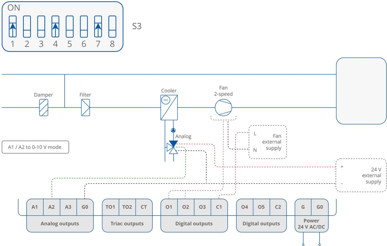
Figure 56. 2-pipe installation with 1-stage analog controlled cooling and 2-speed fan - valve in analog mode
