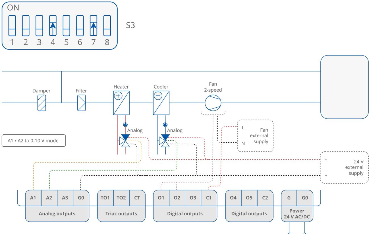
Figure 44. 4-pipe installation with 1-stage analog controlled heating and cooling and 2-speed fan - valve in analog mode
