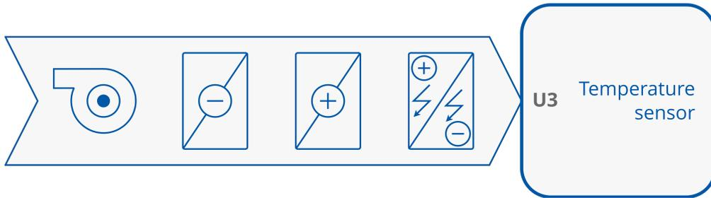
Figure 21. Temperature sensor connected to S3 as a temperature control value source
