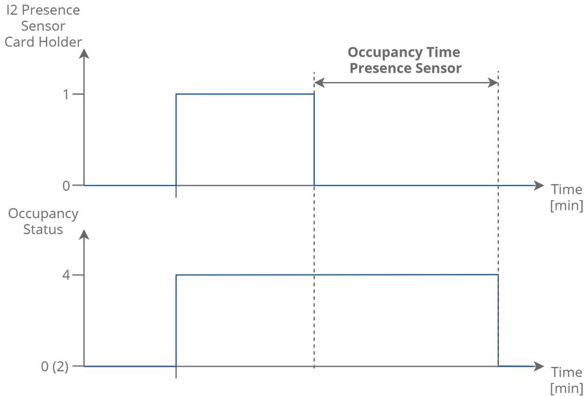
Figure 29. Presence sensor or card holder function time
