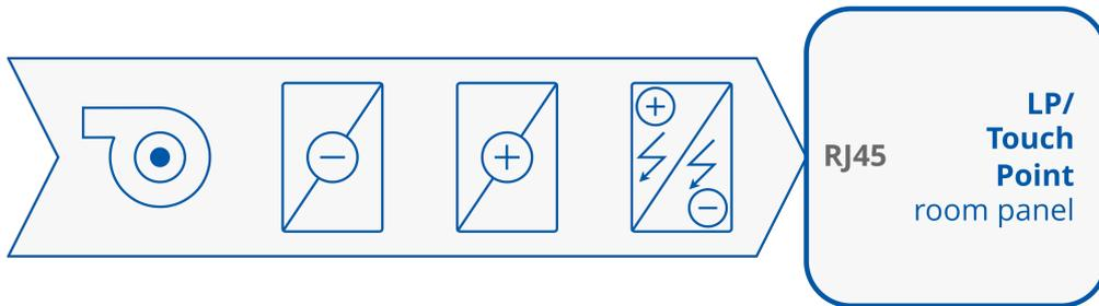
Figure 20. LP/Touch Point room panel set as a temperature source
