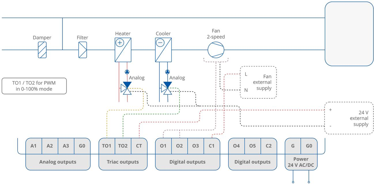
Figure 45. 4-pipe installation with 1-stage analog controlled heating and cooling and 2-speed fan - valve in PWM mode
