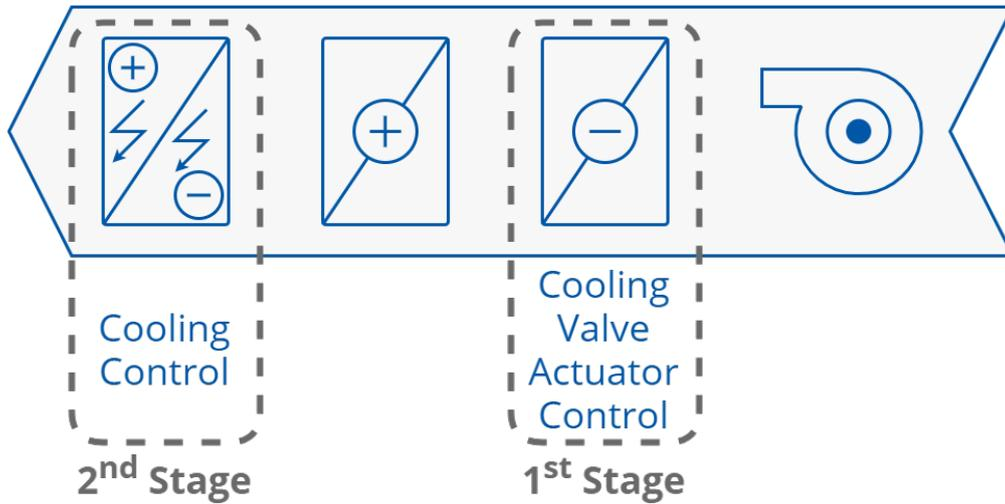
Figure 17. 2 stages of cooling in 2-pipe FCU installation
