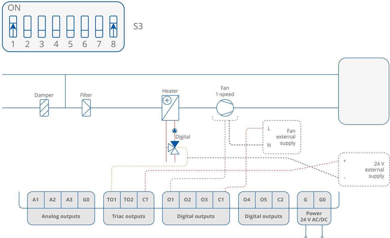
Figure 49. 2-pipe installation with 1-stage digital controlled heating and 1-speed fan
