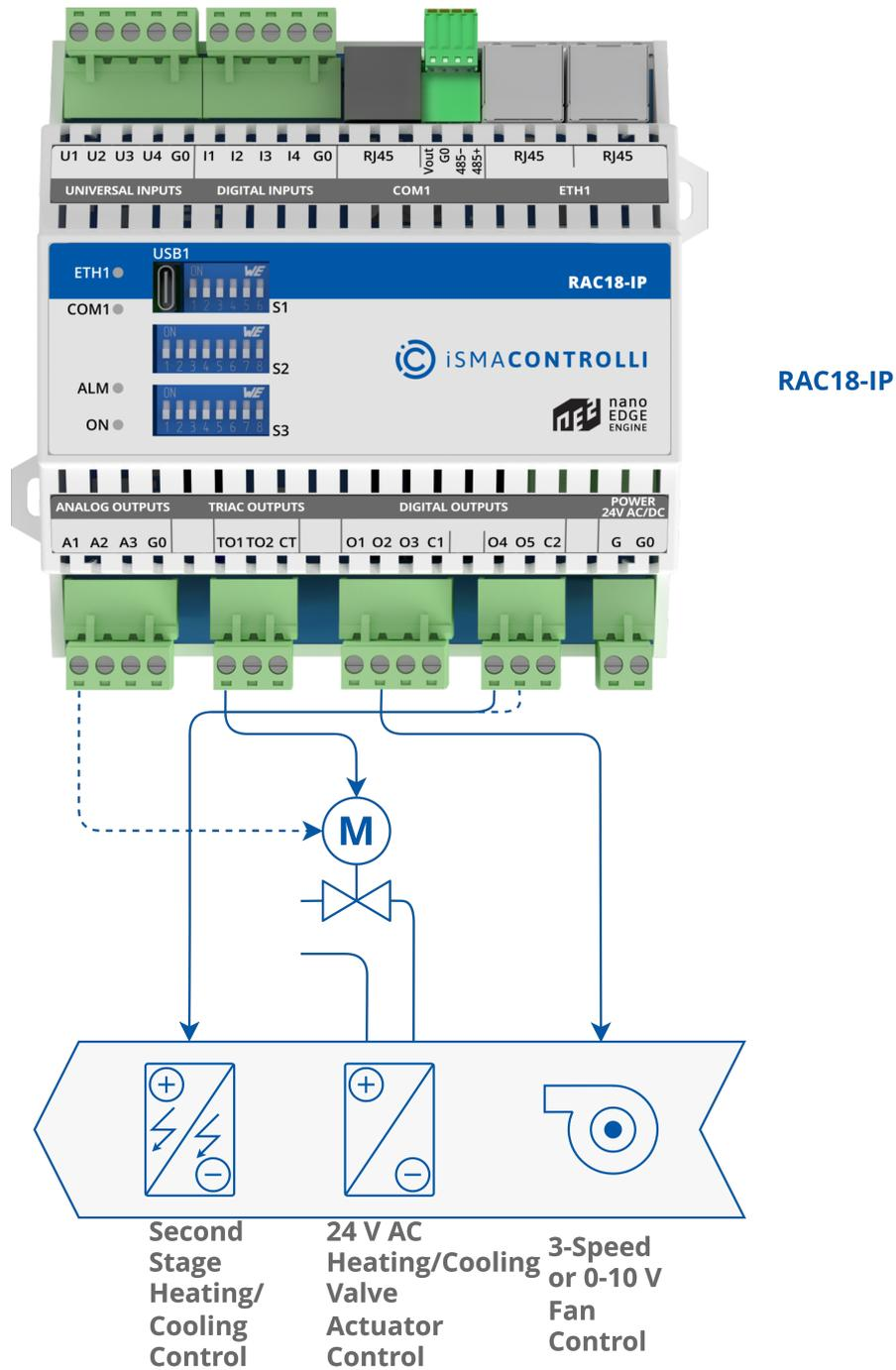
Figure 25. 2-pipe FCU installation
