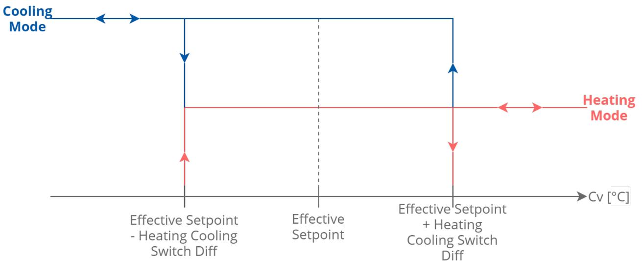
Figure 30. Switching between heating/cooling chart
