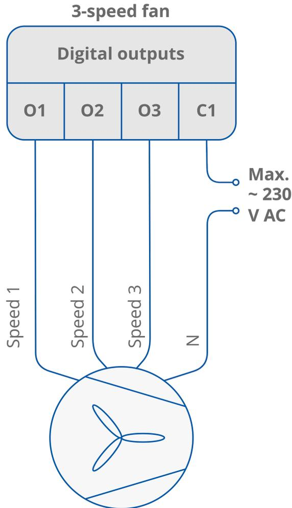
Figure 16. 3-speed fan connection
