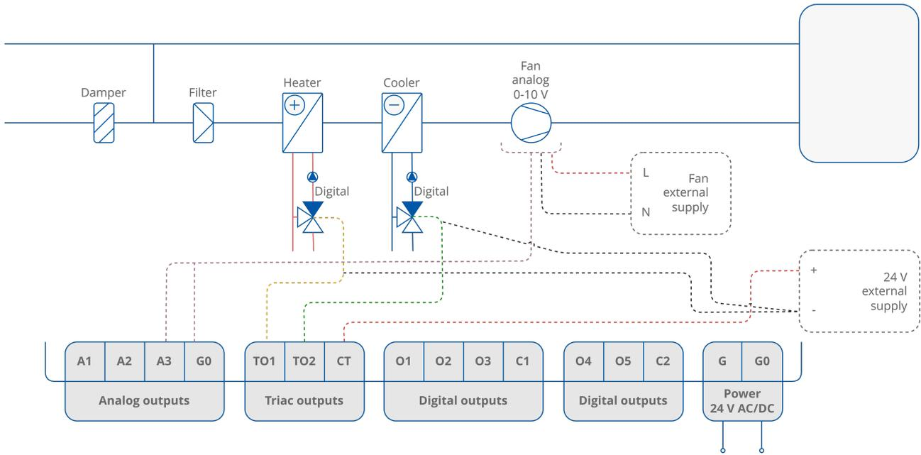
Figure 36. 4-pipe installation with 1-stage digital controlled heating and cooling and analog controlled fan
