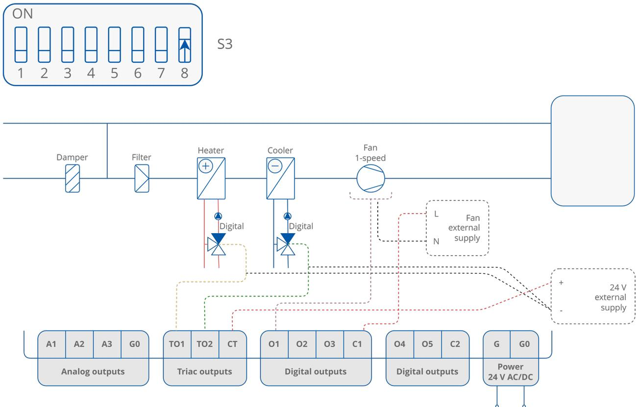
Figure 37. 4-pipe installation with 1-stage digital controlled heating and cooling and 1-speed fan
