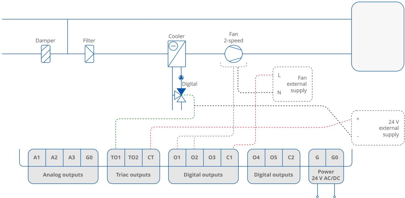
Figure 50. 2-pipe installation with 1-stage digital controlled cooling and 2-speed fan
