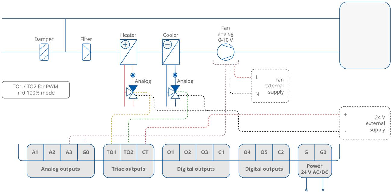
Figure 41. 4-pipe installation with 1-stage analog controlled heating and cooling and analog controlled fan - valve in PWM mode
