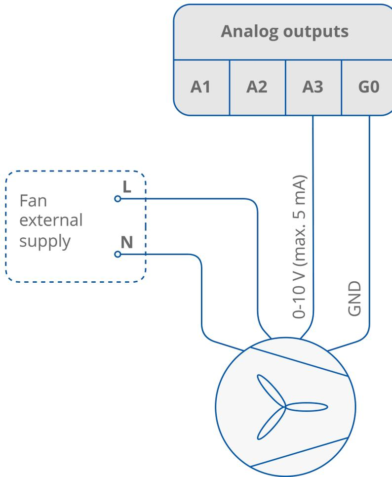
Figure 13. Analog controlled fan connection
