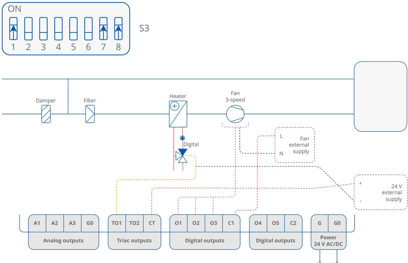
Figure 51. 2-pipe installation with 1-stage digital controlled heating and 3-speed fan
