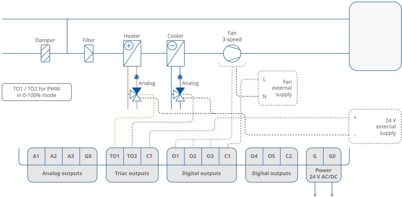
Figure 47. 4-pipe installation with 1-stage analog controlled heating and cooling and 3-speed fan - valve in PWM mode
