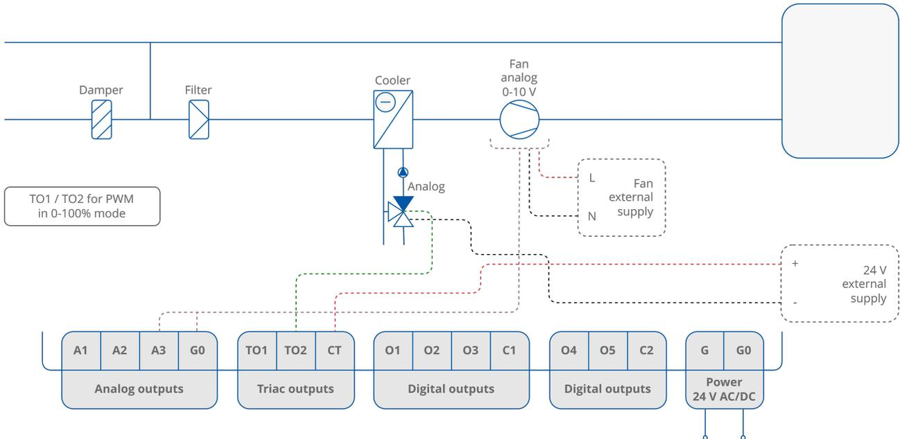
Figure 53. 2-pipe installation with 1-stage analog controlled cooling and analog controlled fan - valve in PWM mode
