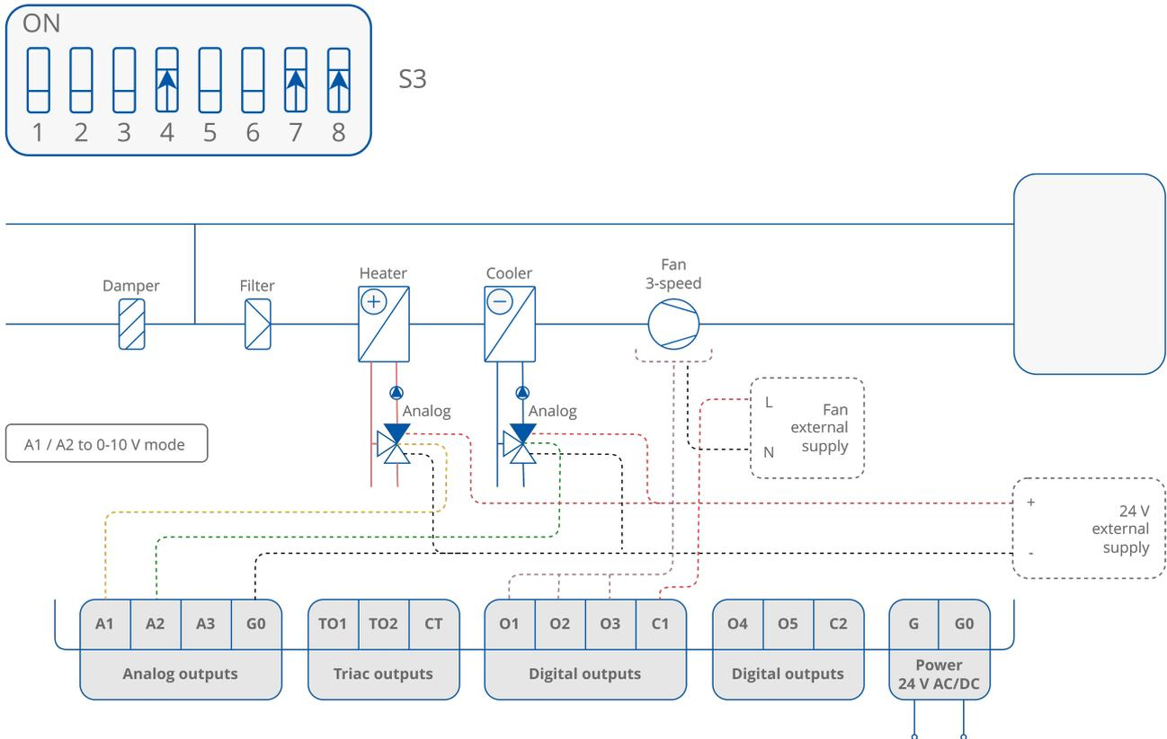
Figure 46. 4-pipe installation with 1-stage analog controlled heating and cooling and 3-speed fan - valve in analog mode
