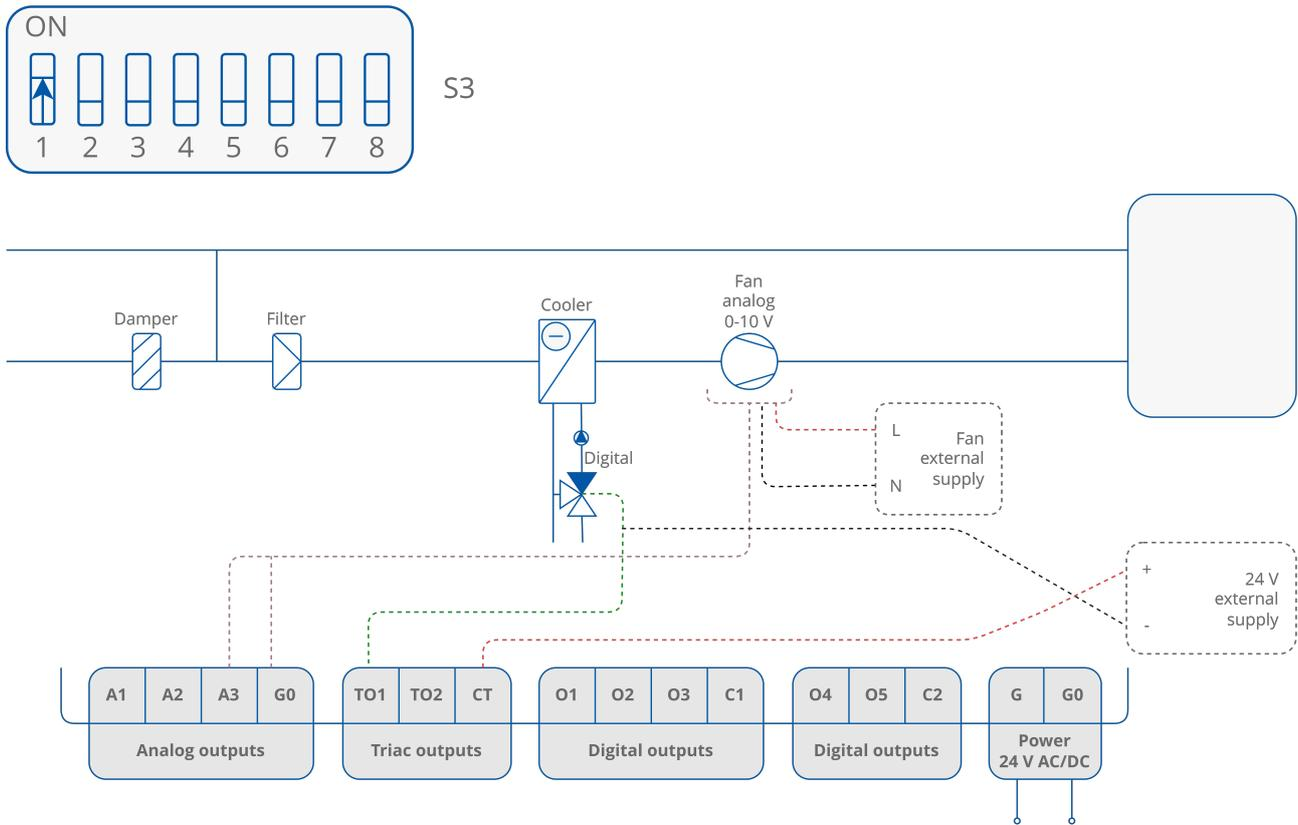
Figure 48. 2-pipe installation with 1-stage digital controlled cooling and analog controlled fan
