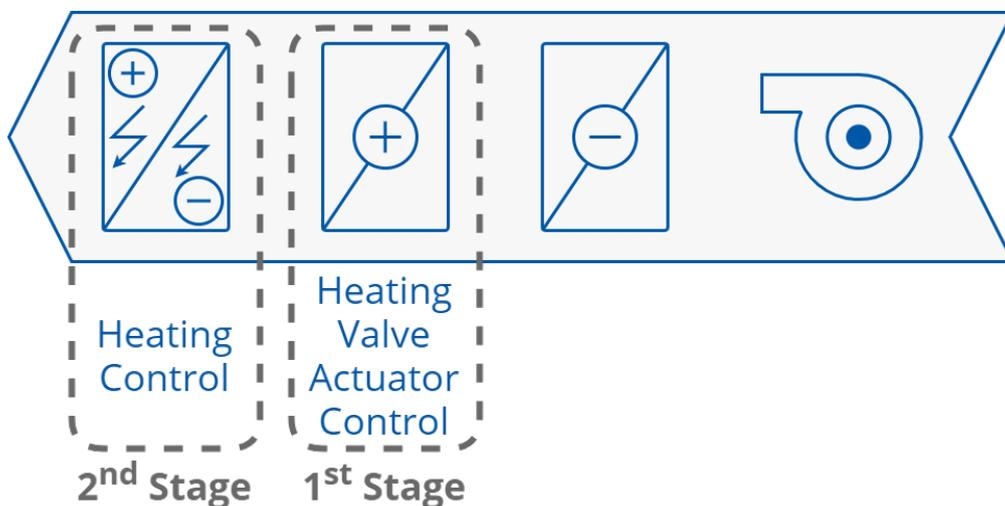
Figure 18. 2 stages of heating in 4-pipe FCU installation
