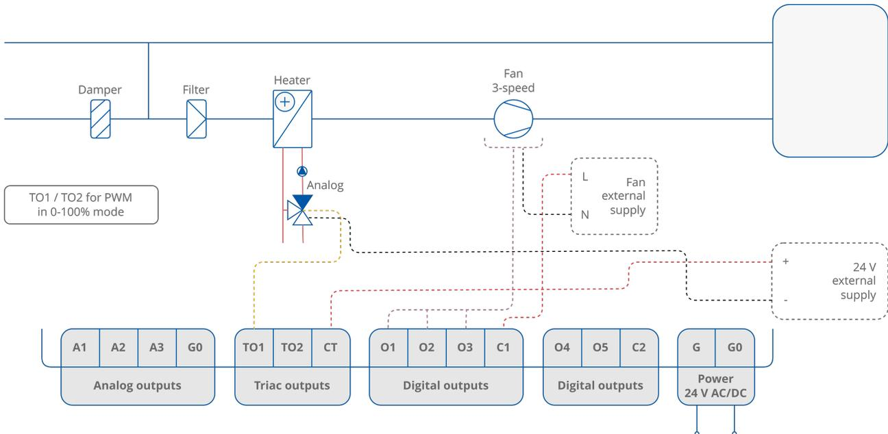
Figure 59. 2-pipe installation with 1-stage analog controlled heating and 3-speed fan - valve in PWM mode
