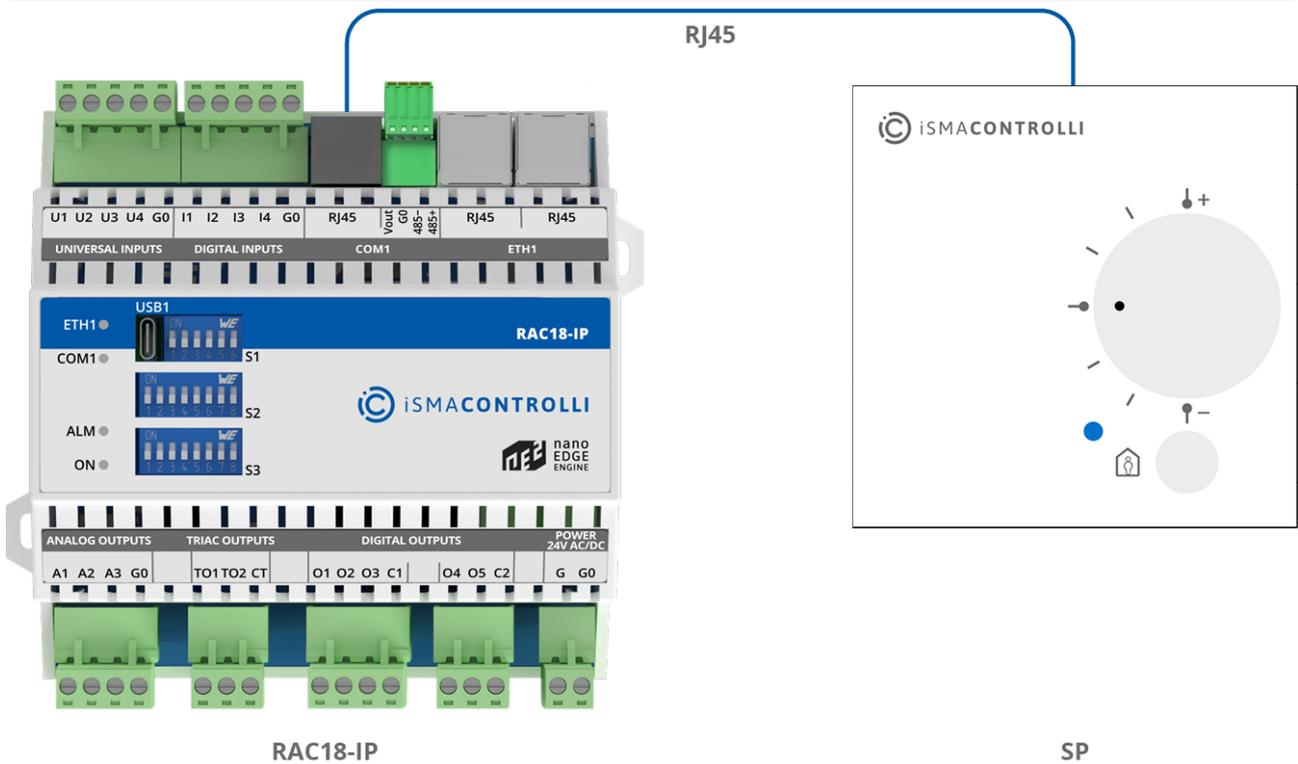
Figure 33. RAC18-IP connection to SP panel
