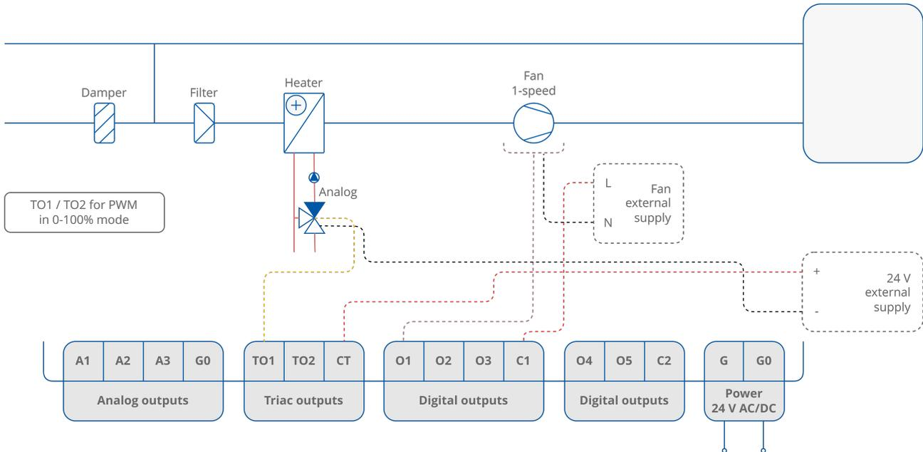
Figure 55. 2-pipe installation with 1-stage analog controlled heating and 1-speed fan - valve in PWM mode
