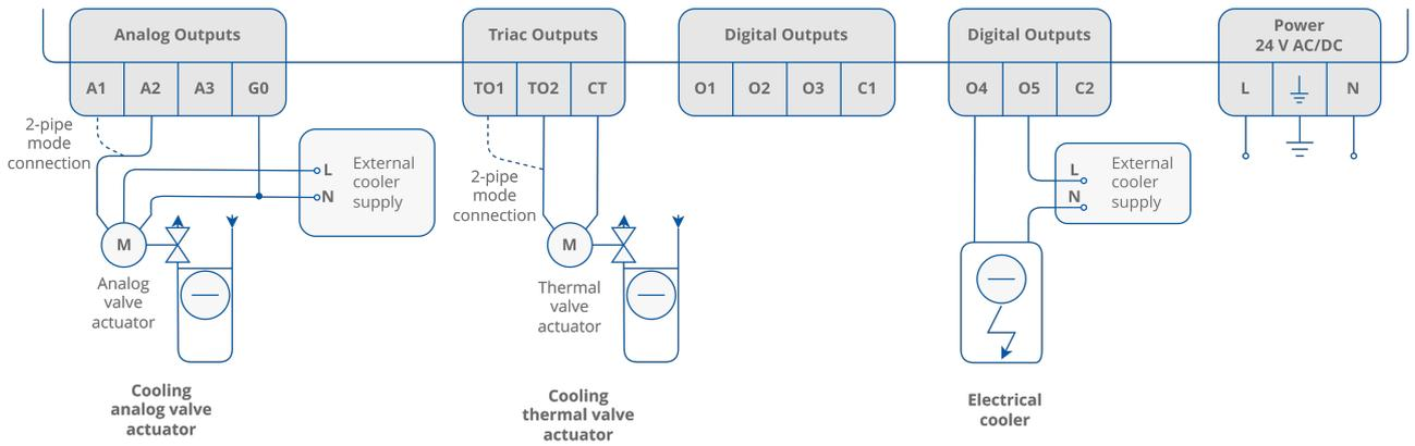
Figure 27. Cooling actuators connection
