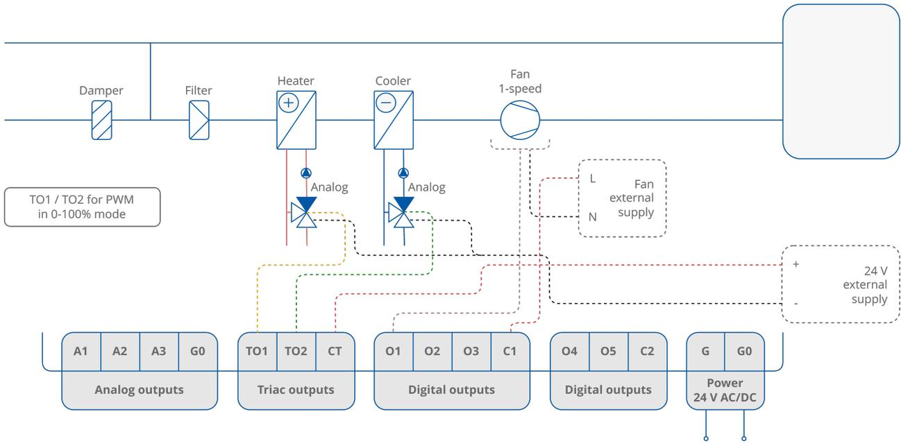
Figure 43. 4-pipe installation with 1-stage analog controlled heating and cooling and 1-speed fan - valve in PWM mode
