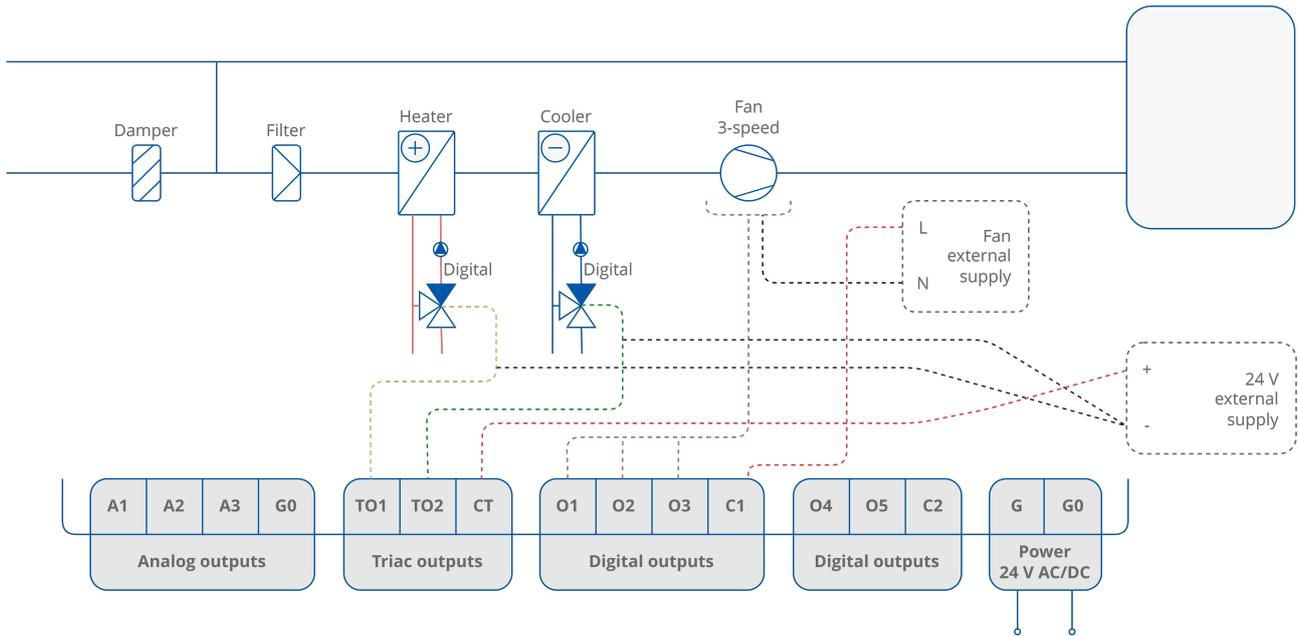
Figure 39. 4-pipe installation with 1-stage digital controlled heating and cooling and 3-speed fan
