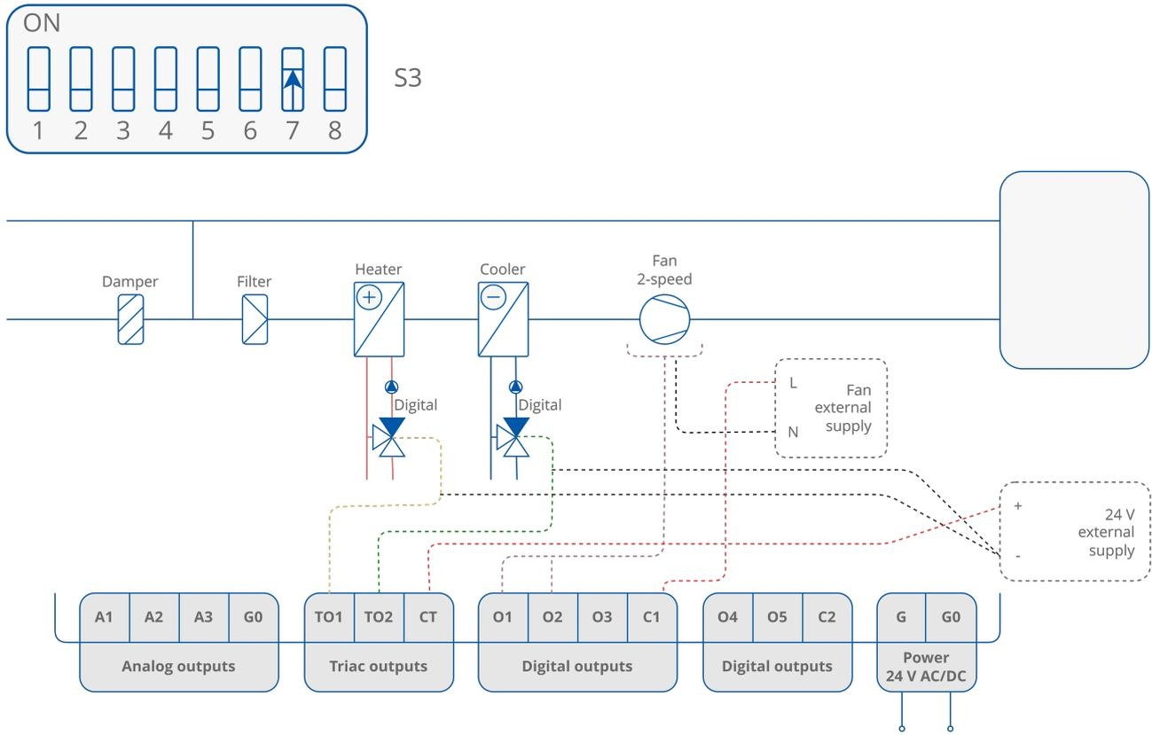
Figure 38. 4-pipe installation with 1-stage digital controlled heating and cooling and 2-speed fan
