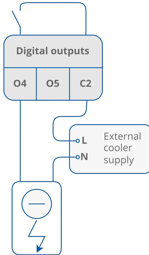
Figure 7. Electrical cooler connection
