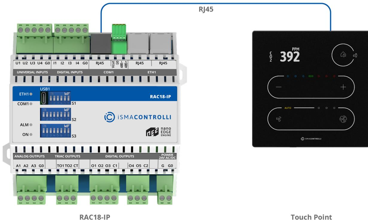
Figure 31. RAC18-IP connection to Touch Point panel
