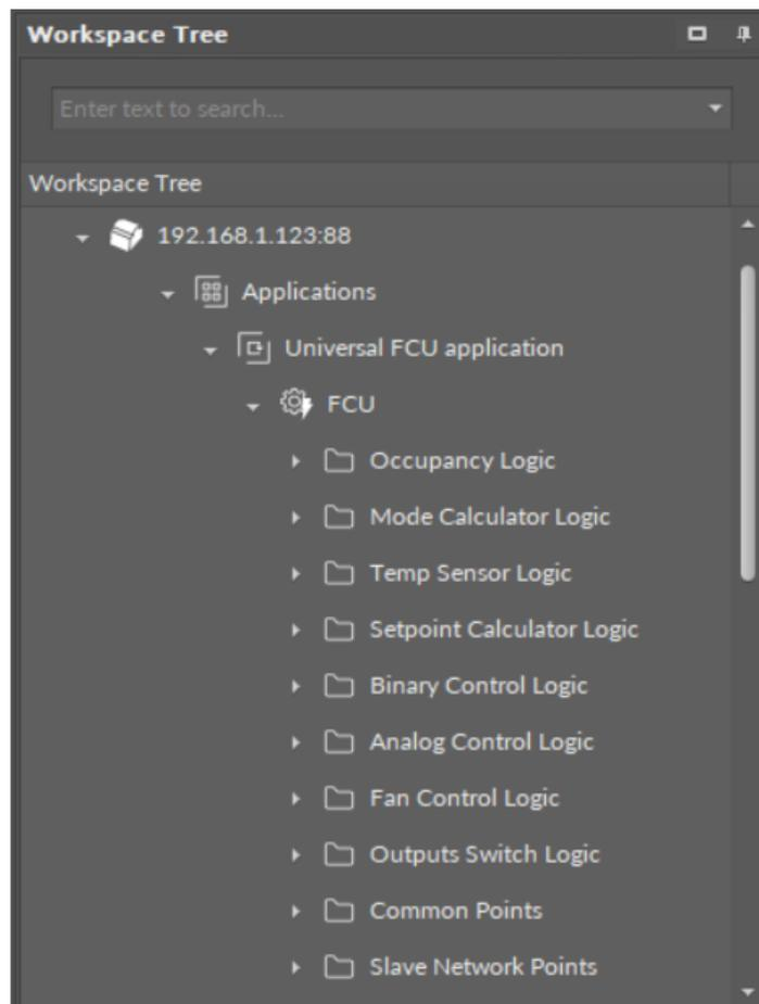
Figure 1. Universal FCU application in the iC Tool
