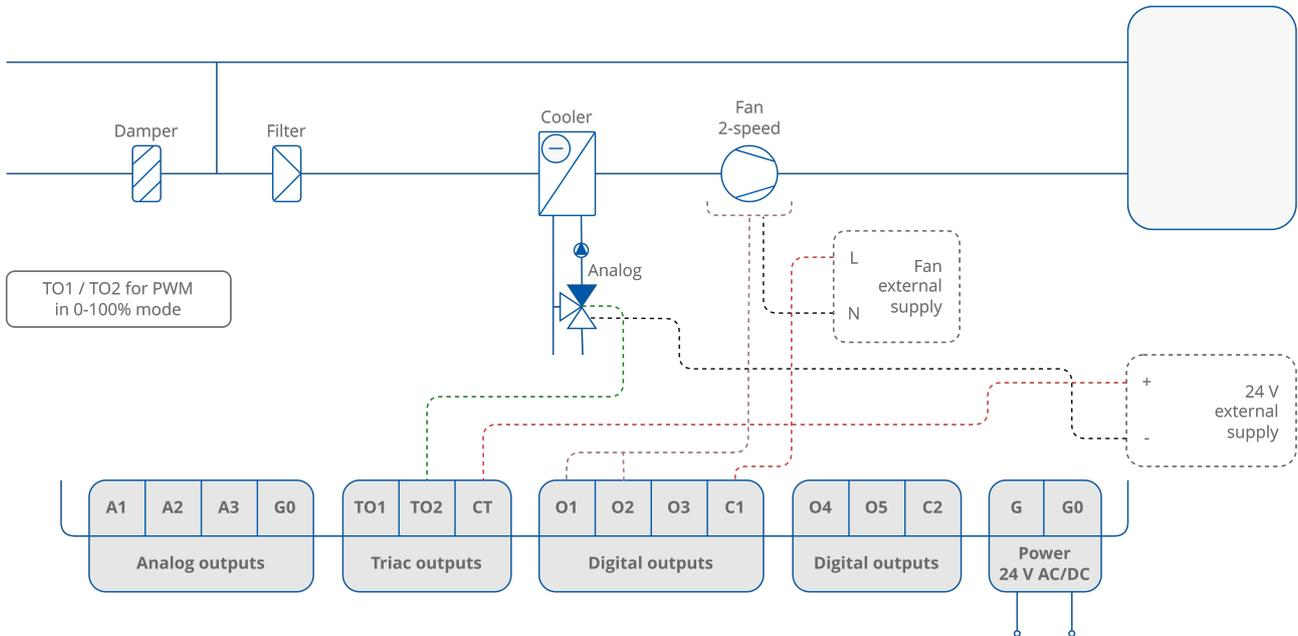
Figure 57. 2-pipe installation with 1-stage analog controlled cooling and 2-speed fan - valve in PWM mode
