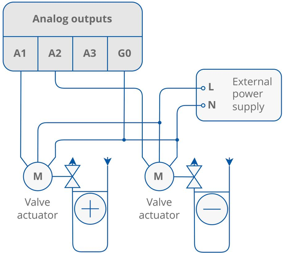
Figure 8. Connection of analog valve actuators
