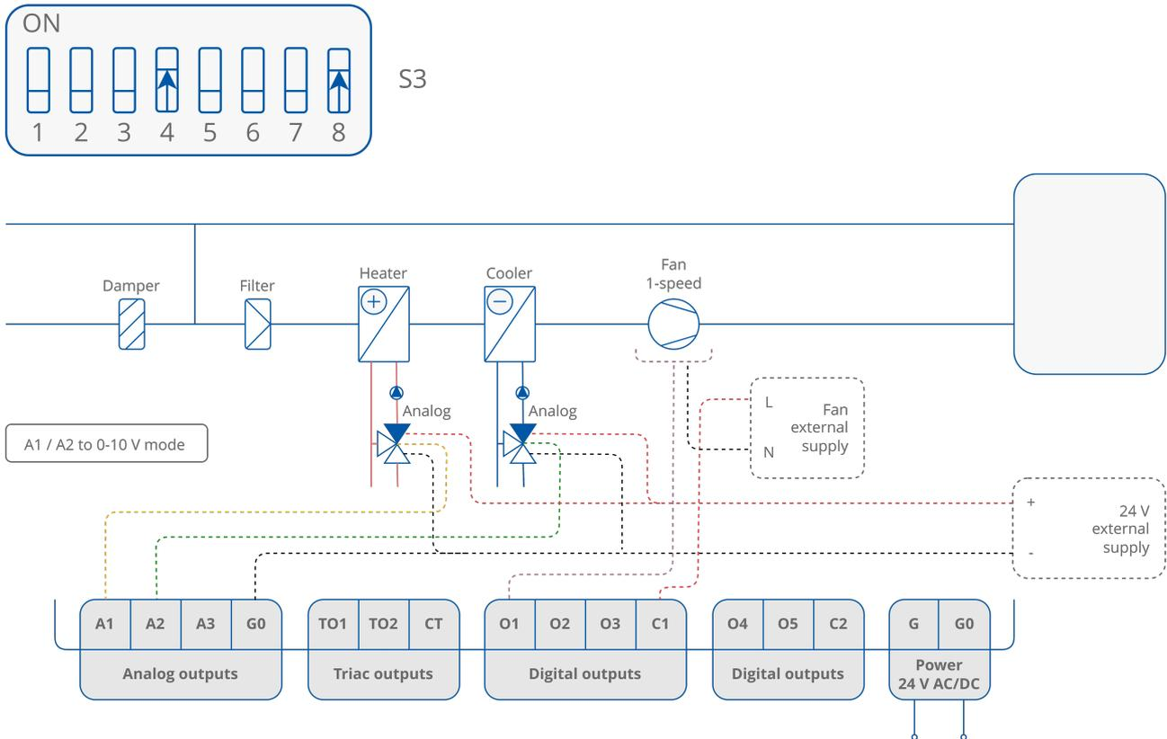
Figure 42. 4-pipe installation with 1-stage analog controlled heating and cooling and 1-speed fan - valve in analog mode
