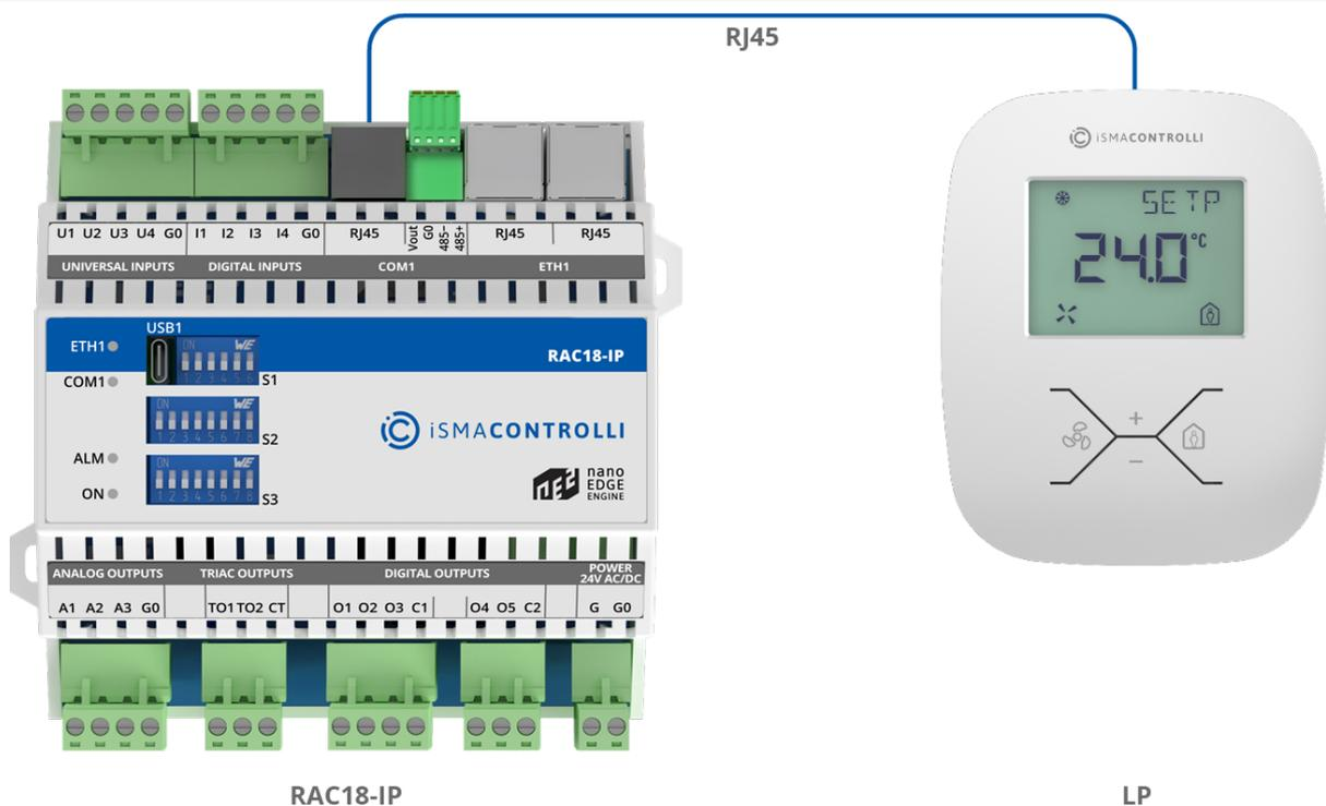
Figure 32. RAC18-IP connection to the LP pane
