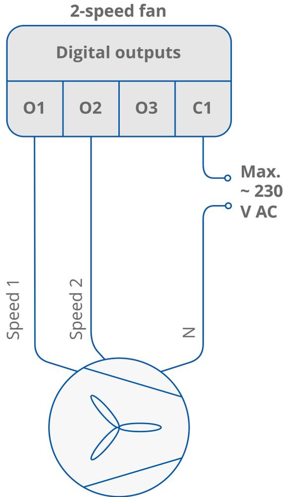
Figure 15. 2-speed fan connection
