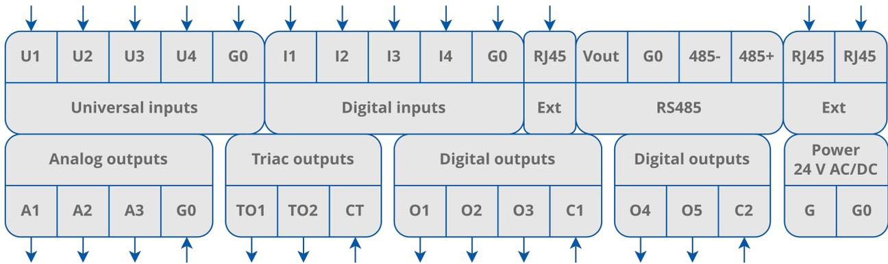
Figure 35. Inputs and outputs overview
