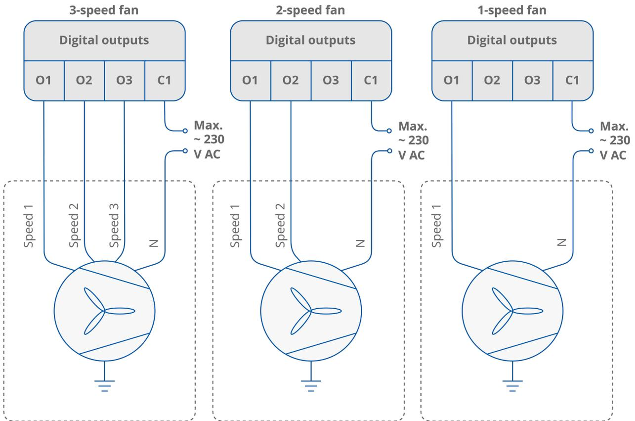
Figure 5. Fan connections
