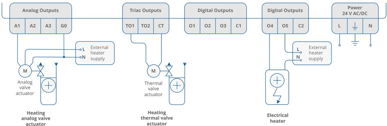
Figure 26. Heating actuators connection
