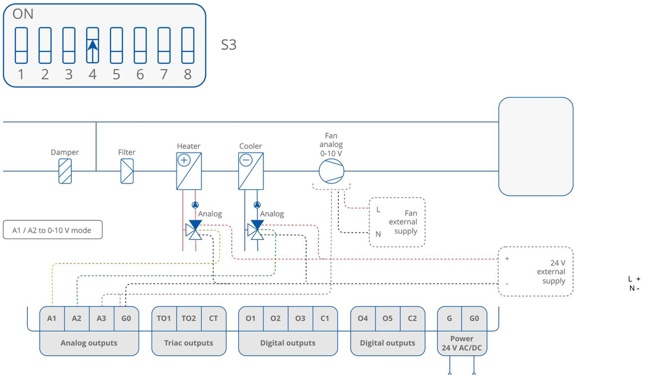
Figure 40. 4-pipe installation with 1-stage analog controlled heating and cooling and analog controlled fan - valve in analog mode
