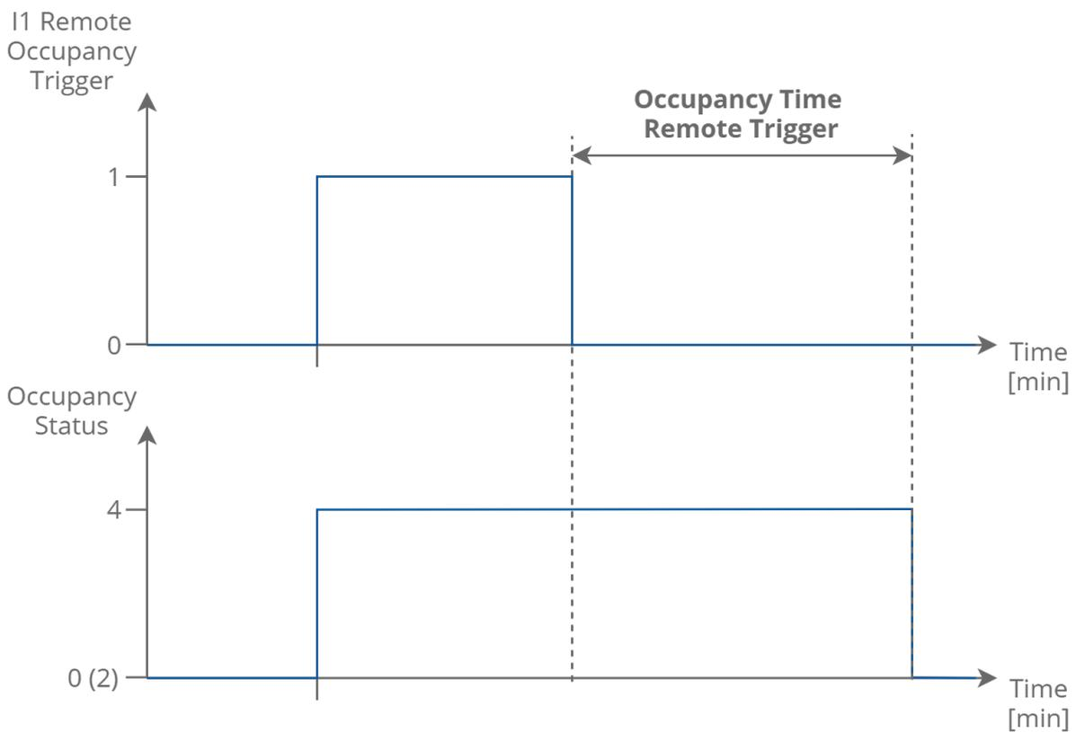
Figure 28. Occupancy trigger time function
