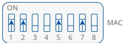
Figure 13. MAC DIP switch settings
