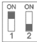
Figure 12. Position of the DIP switch no. 1 for restoring default settings
