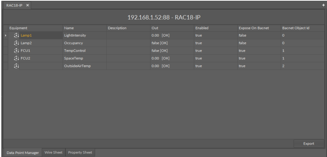
Figure 23. The Data Point Manager for the RAC18-IP BACnet LocalDevice
