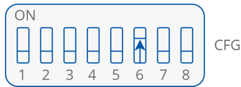
Figure 26. On/Off light control configuration
