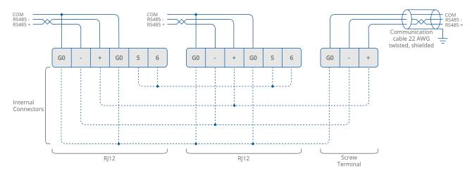
Figure 9. Internal connections between RJ12 sockets and a main RS485 socket
