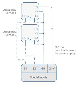
Figure 18. Special inputs connection
