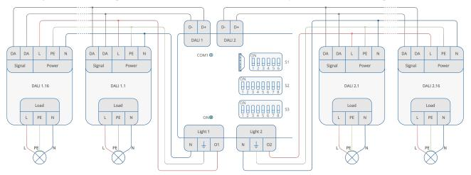
Figure 17. Connection and ballasts and lamps to the device
