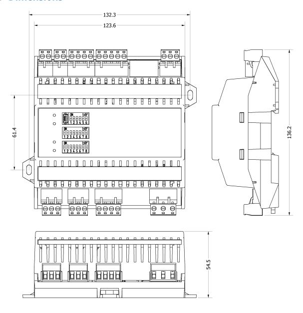
Figure 1. Dimensions of iSMA-B-2D
