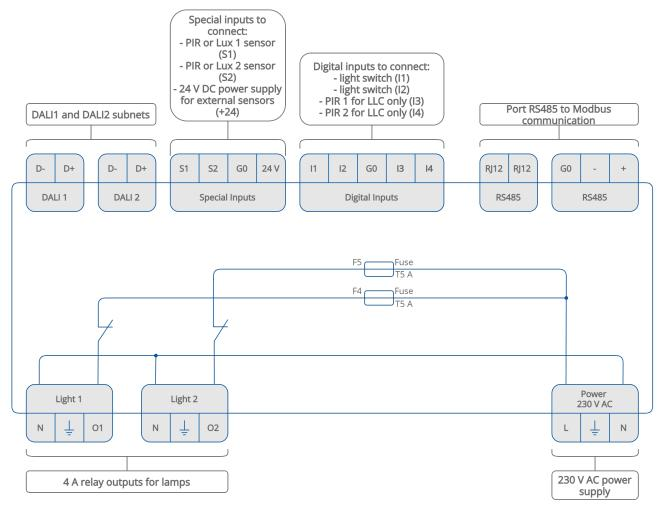
Figure 6. iSMA-B-2D-WD terminals and internal connections
