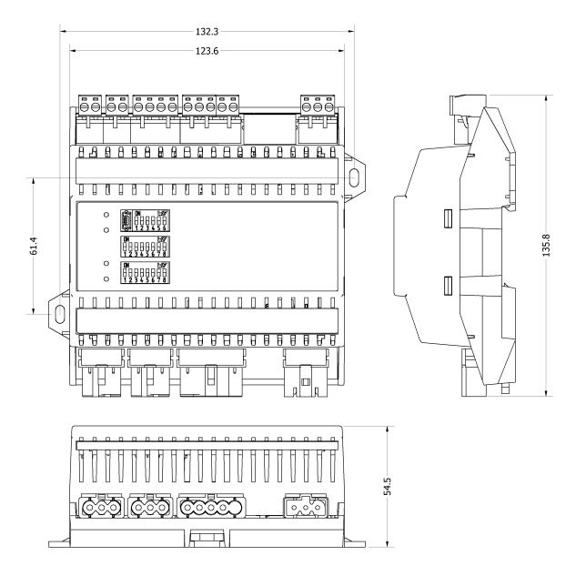
Figure 2. Dimensions of iSMA-B-2D-WD
