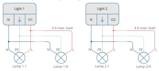
Figure 22. Connecting lamps to light outputs in the On/Off control mode
