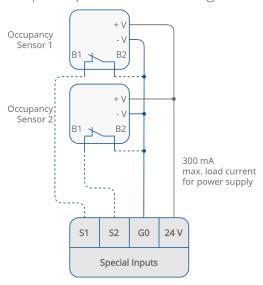
Figure 23. Example of connecting sensors to 24 V DC power supply outputs
