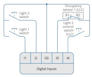
Figure 33. The light 2 control switch connected to 14
