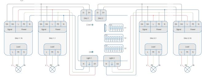
Figure 21. Connecting ballasts to light outputs in the DALI control mode
