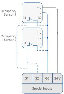
Figure 4. 24 V DC power supply connection
