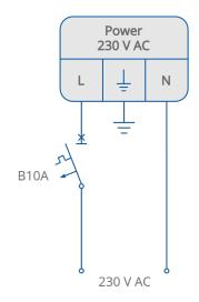
Figure 3. 230 V AC power supply connection
