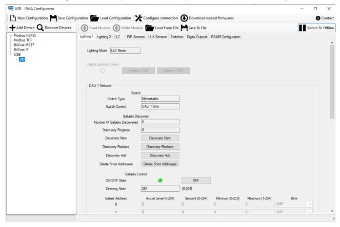
Figure 34. Lighting tabs 1 and 2 for devices working in the LLC mode
