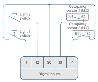
Figure 32. Switches and sensors connected to digital inputs
